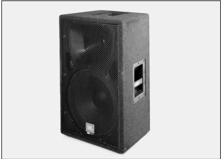
reinforcement of speech. The Laminar Flow Baffle reduces diffraction effects and distortion resulting from turbulence. The horn design with its large mouth delivers smooth, natural reproduction - especially in the critical mid-range. The edges of the premium grade carpet are captured by the joint detail to prevent visible seams or peeling. A 16 gauge, steel grill protects the 15 inch JBL woofer.
